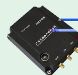
⑦ Partial discharge online monitoring module
